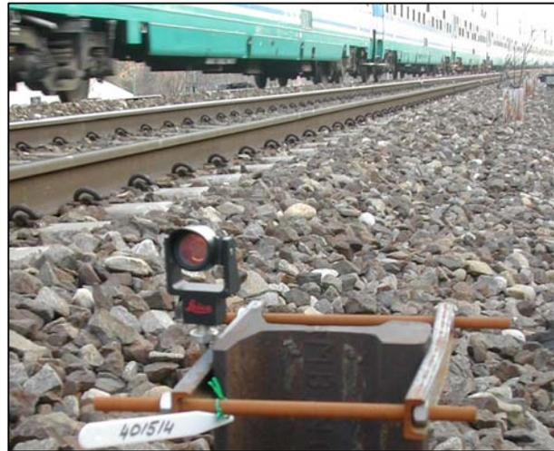
Figure 5 – Prism on railway embankment pedestal
