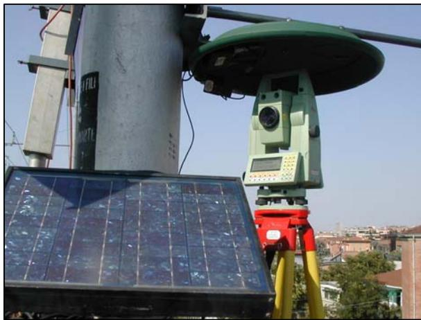
Figure 6 – Total station installation
