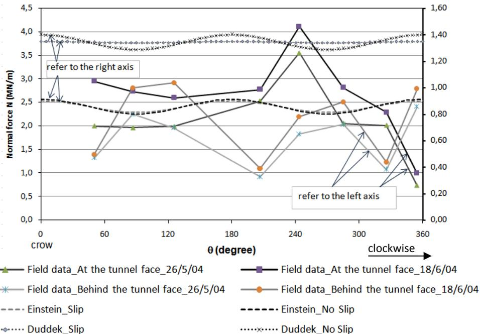
Figure 6 Normal force diagram in the lining ring 582
