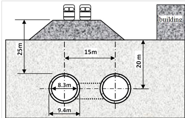
Figure 1 Typical cross-section of the two tunnels excavated below the railway
