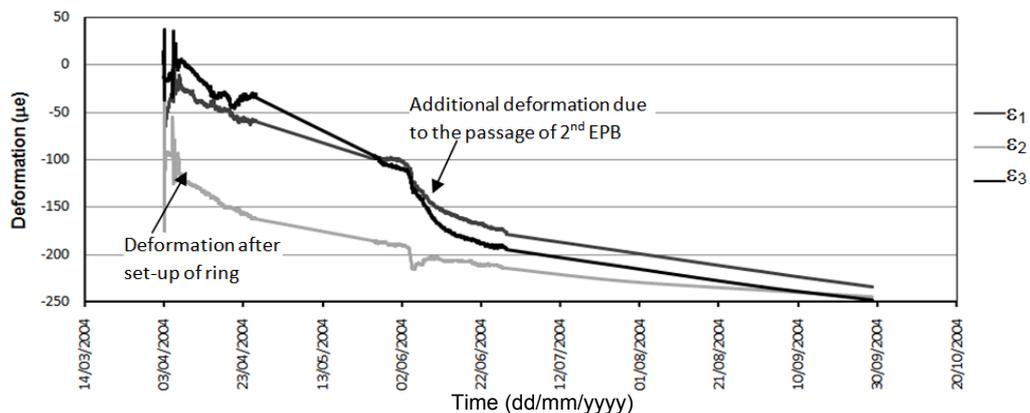
Figure 4 Deformation with time of the ring 582 - block A1
