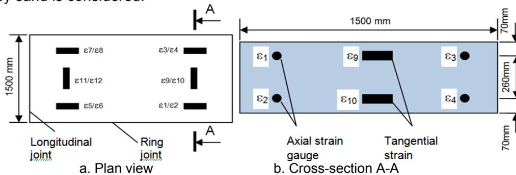
Figure 3 Layout of strain gauges in odd blocks (not scaled)
