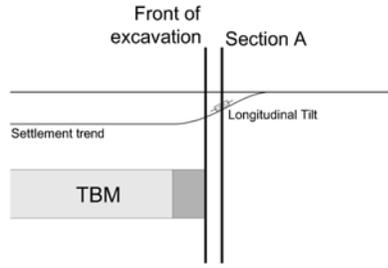
Figure 14. Longitudinal section next to excavation front
