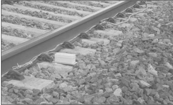
Figure 6. Transversal electrolevel
