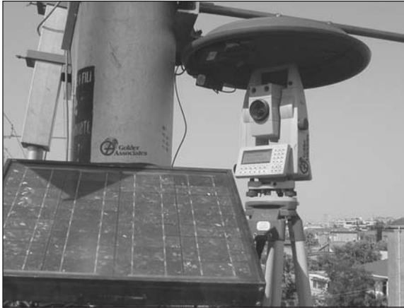
**Figure 8. Typical TS installation**
