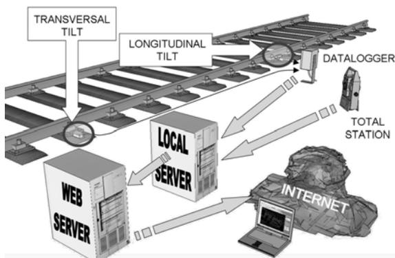
Figure 10. Hardware configuration of monitoring system
