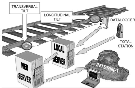
Figure 10. Hardware configuration of monitoring system
