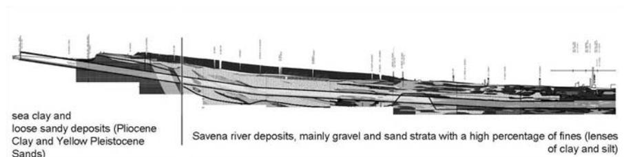
Figure 2. Geological section along rail track
