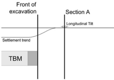
Figure 13. Longitudinal section undisturbed
