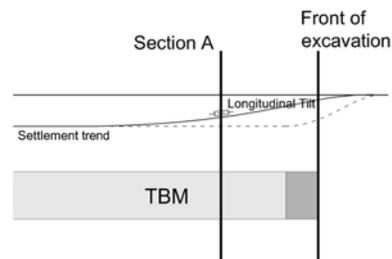
Figure 16. Longitudinal section, case "B"
