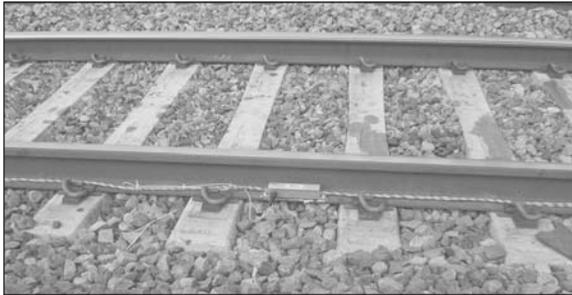
Figure 5. Longitudinal electrolevel
