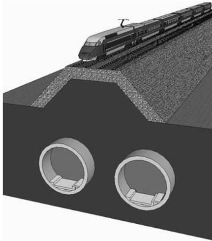
**Figure 3. Cross section of the tunnels under railway embankment**
